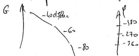
$$\text{du diagramme } \pi \varphi = 180 - 120 = 60^\circ$$
