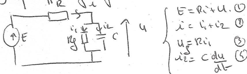
$$\left\{ \begin{array}{l} E = R \cdot i + U \quad (1) \\ i = i_1 + i_2 \quad (2) \\ U = R \cdot i_1 \quad (3) \\ i_2 = C \frac{du}{dt} \quad (4) \end{array} \right.$$
