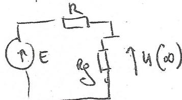
$$U(\infty) = \frac{Rg}{R+Rg} \cdot E \quad \text{si } Rg \gg R \quad Rg + R \rightarrow Rg$$
